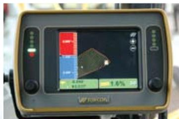
With the Topcon 3D-GPS+ system, job information is uploaded into a control box mounted on the dash of a Komatsu dozer or grader, directly in front of the operator. The operator controls direction and speed, while the 3D-GPS+ system automatically positions the blade to create the finish grade.
