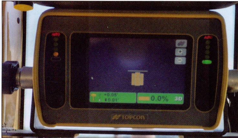
Topcon GPS control box provides data to the equipment operator.
